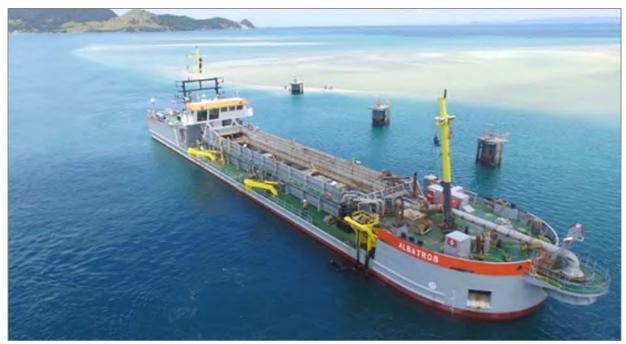
Photo 2 The Albatros trailing suction dredge (photo: <a href="https://www.dutchdredging.nl/">https://www.dutchdredging.nl/</a>)
